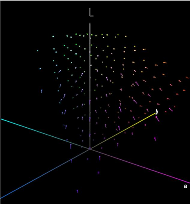
**Figure 4.** CIE Lab vector plot showing reference test color points and how they are reproduced by the color-managed NDS E3cHB LCD.
