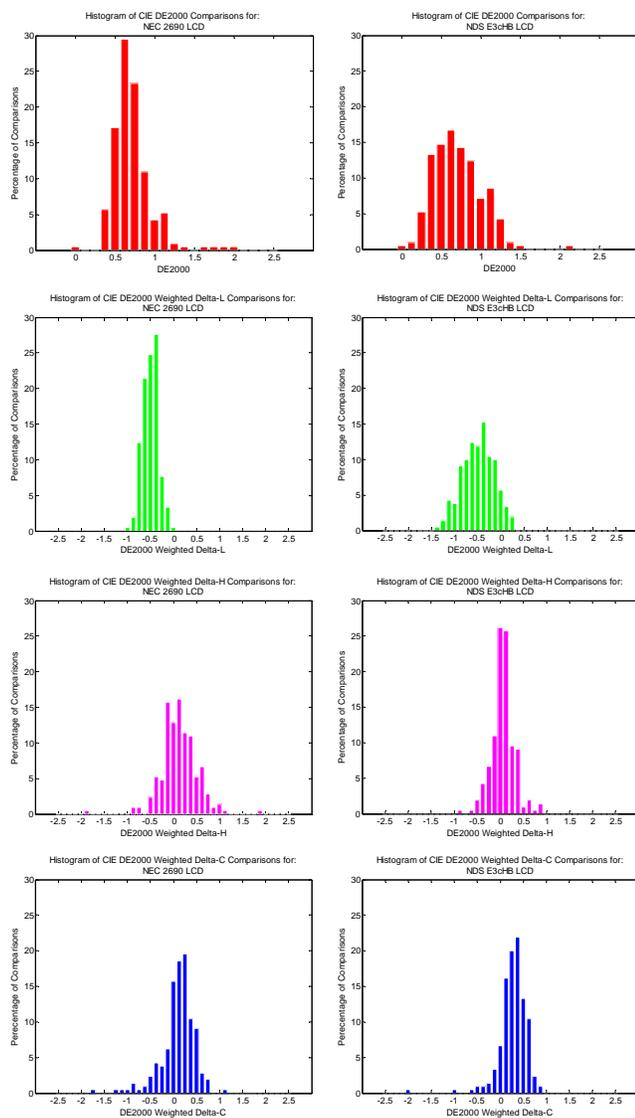
**Figure 3. Histograms of DE2000 color differences, lightness differences, hue-angle differences and chroma differences for the NEC 2690 LCD (left) and NDS E3cHB LCD (right) .**
