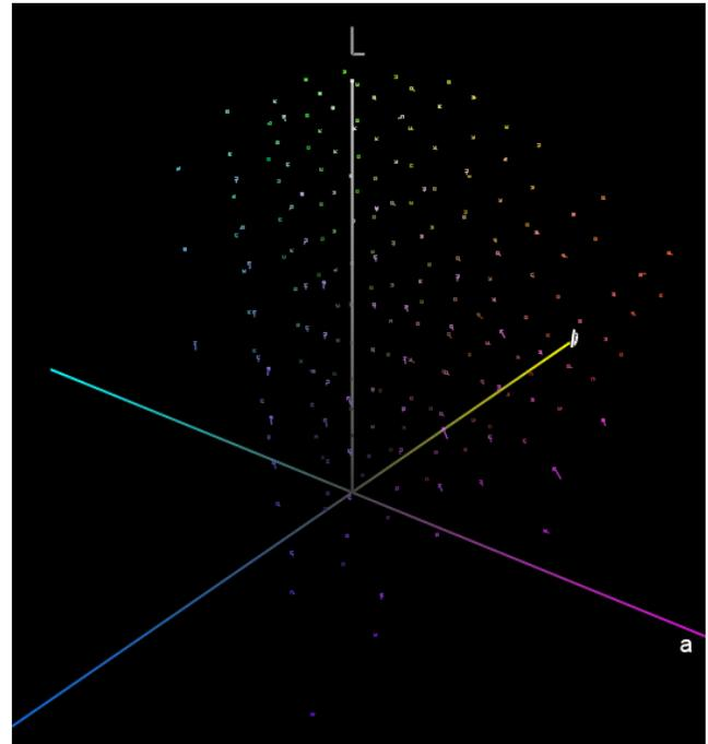
**Figure 2. CIE Lab color vector plot showing reference test color points and how they are reproduced by the color-managed NEC 2690 LCD.**
